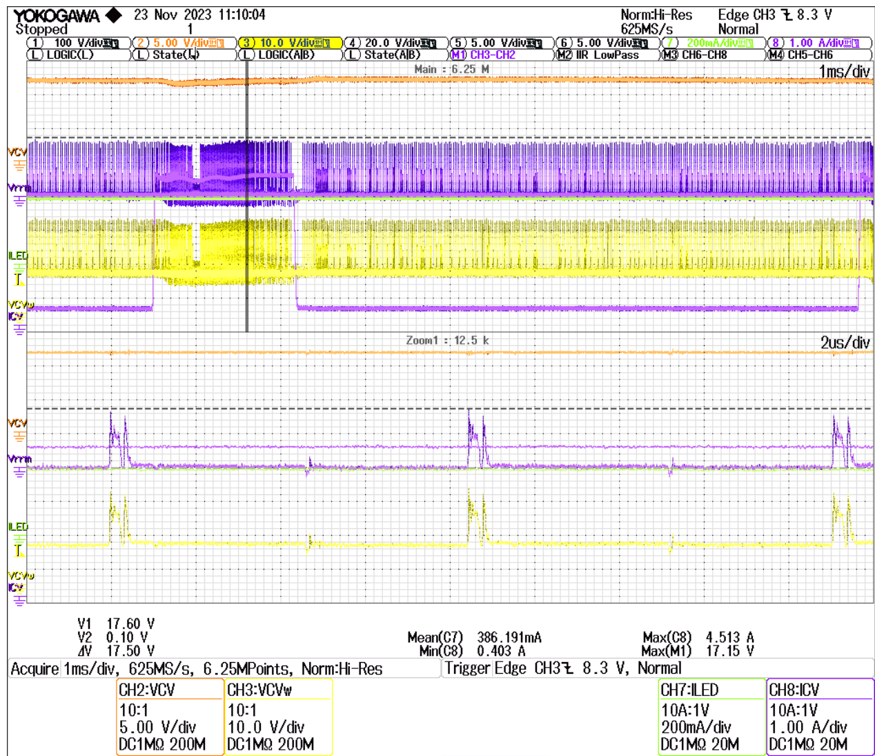
Figure 62 – CV1 Selection FET (Q1) D-S Voltage Under Peak Load at 90 VAC.
