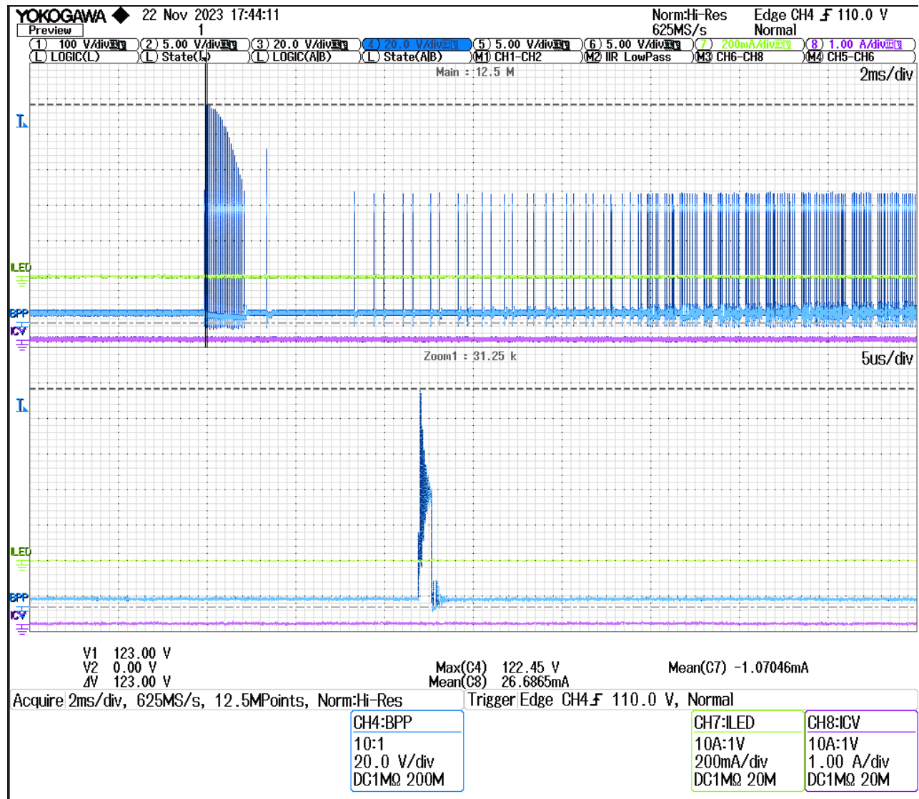
Figure 73 – Auxiliary Diode Reverse Voltage at Start-up at 265 VAC.
